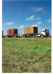
rummed uranium concentrates secured in ISO containers are transported by road train to Darwin for loading aboard ship.
