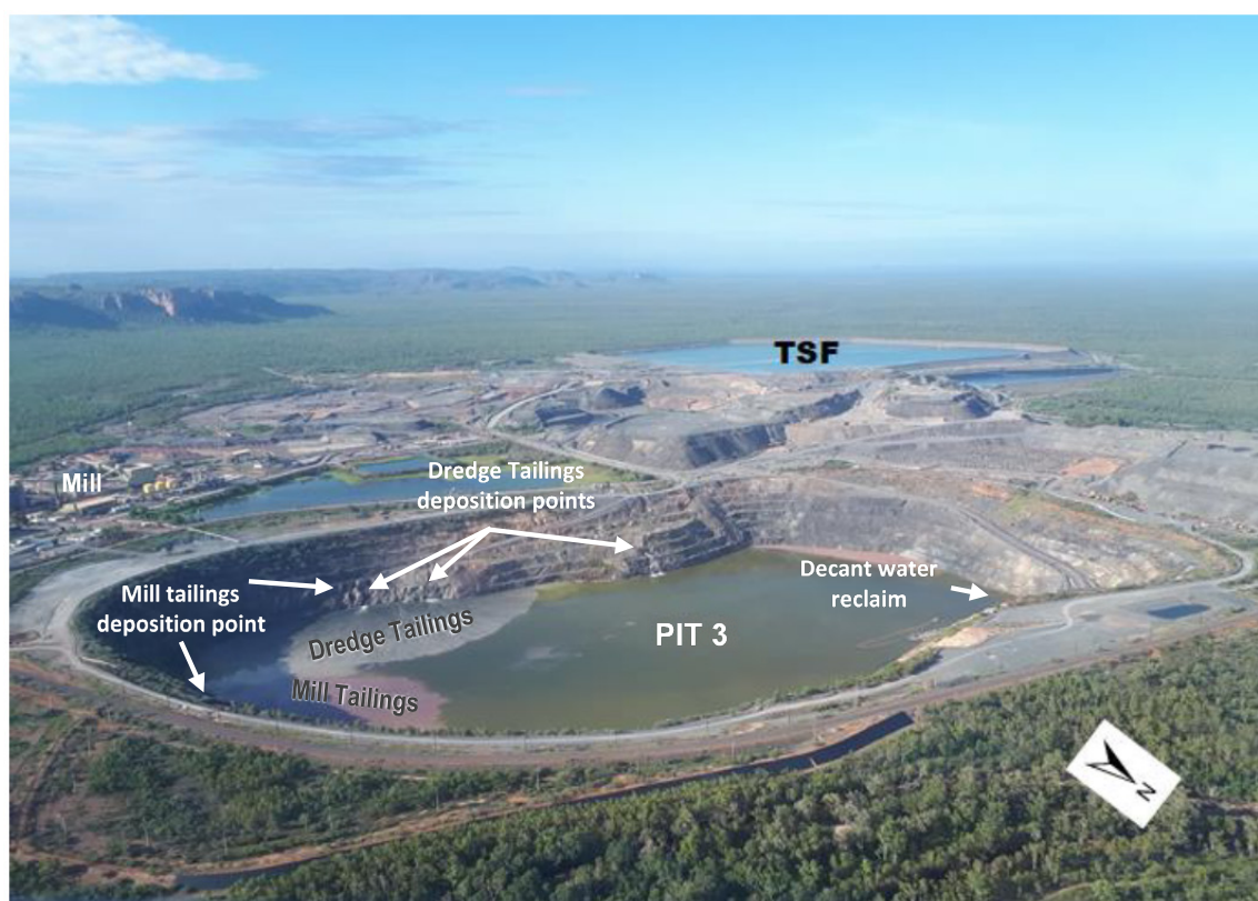
Figure 9-13: Pit 3 showing the original location of mill and dredge tailings deposition points
