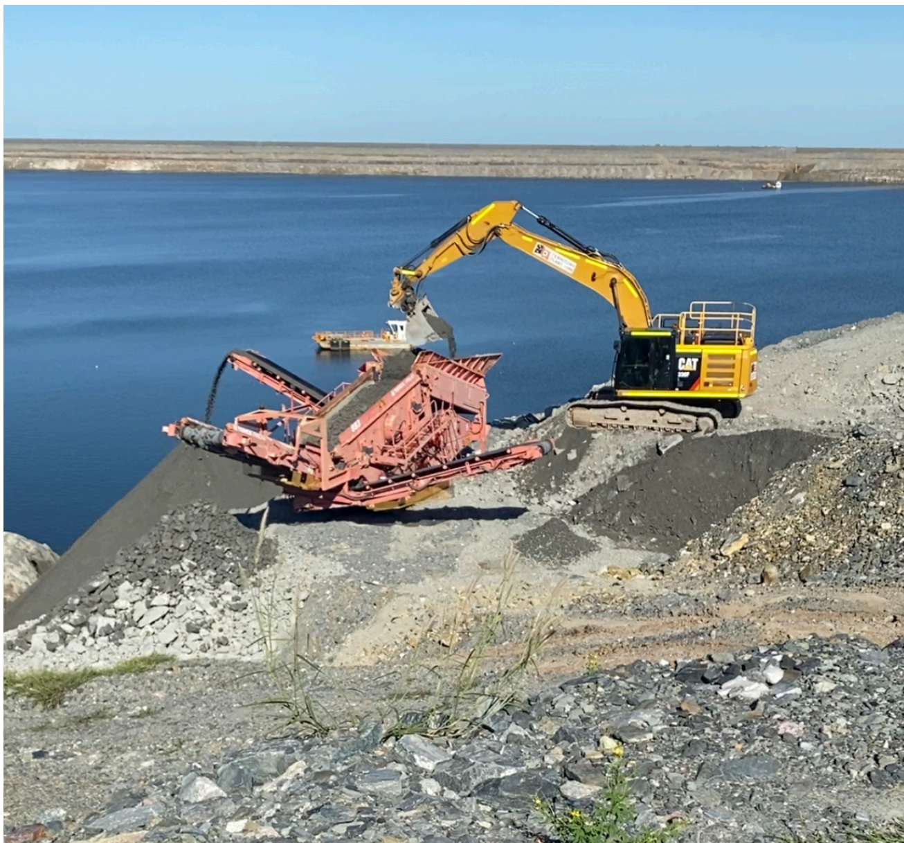
Figure 9-33: Sorter/stacker removing rocks before placing tailings into dredge pool.
