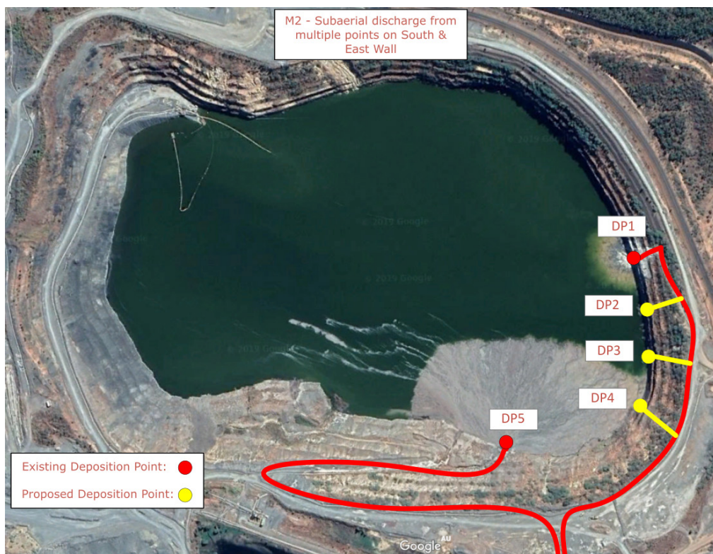
Figure 9-16: Subaerial deposition of mill tailings from multiple spigot points
