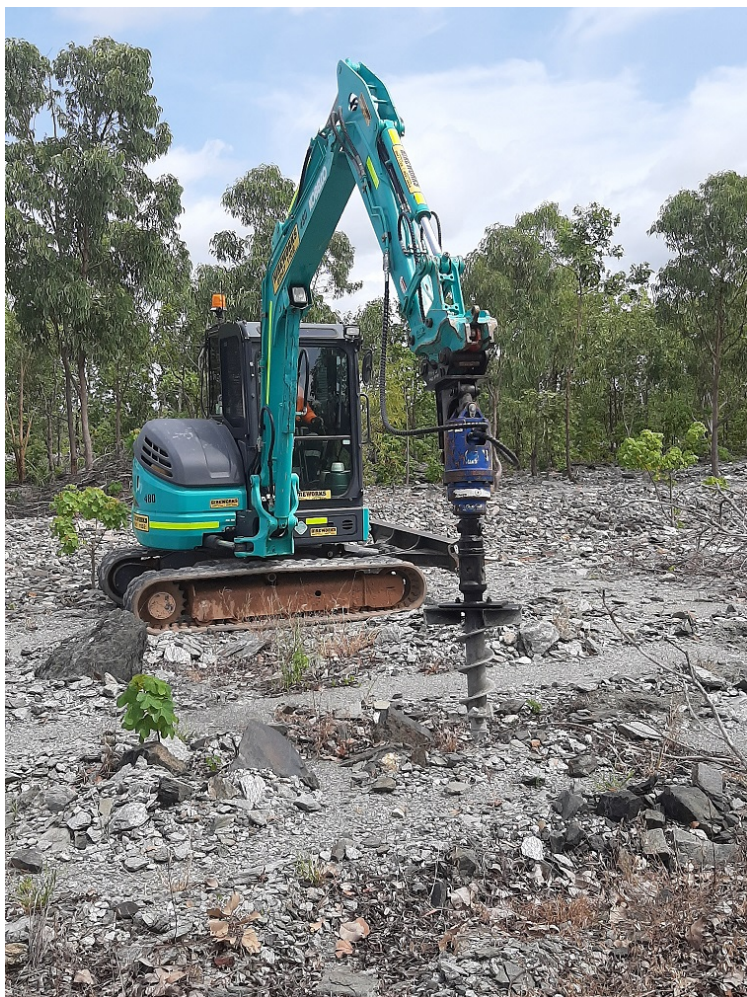
Figure 9-96: Example of a specially modified auger cultivator attached to a small excavator, here seen being trialed in waste rock on the Trial Landform in March 2020.
