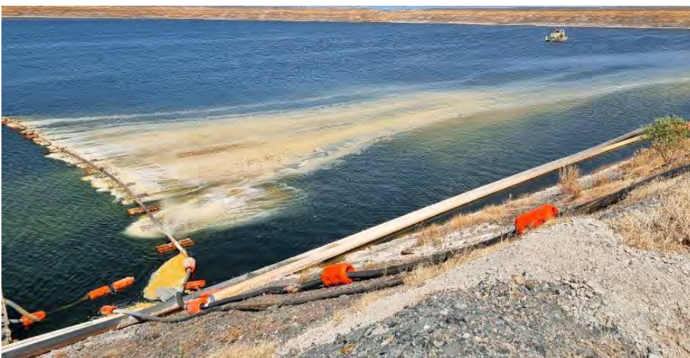
Photo 4-27: Limestone dosing to raise pH of the RWD water
