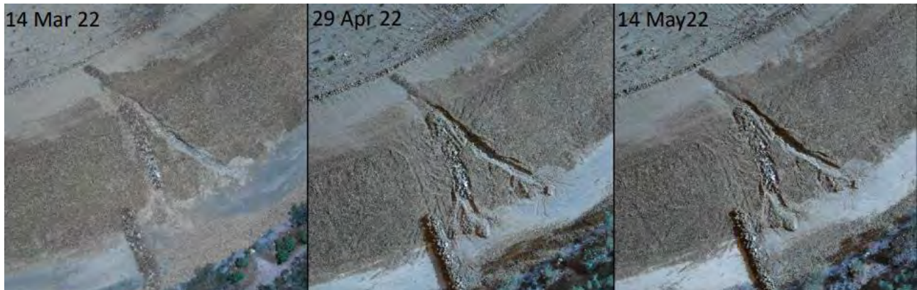
Photo 4-7: Back-cutting erosion on the steeper slope leading into the temporary perimeter drain (2022)
