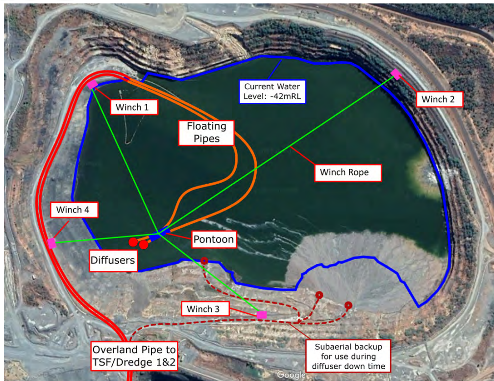
Figure 9-24: Subaqueous deposition of dredge tailings via floating pipelines and diffusers
