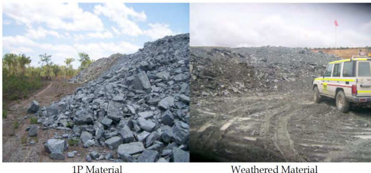
Figure 9-103: Rock types used to construct the trial landform
