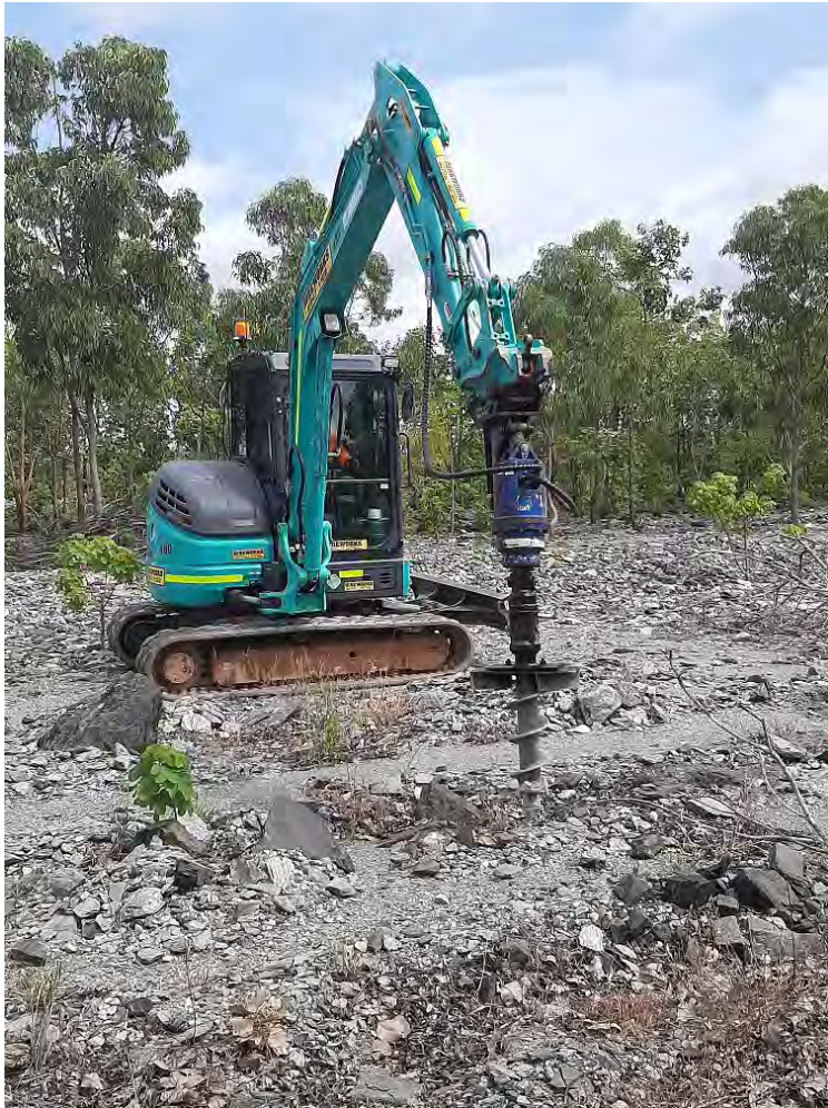
Figure 9-124: Example of a specially modified auger cultivator attached to a small excavator, here seen being trialled in waste rock on the Trial Landform in March 2020.
