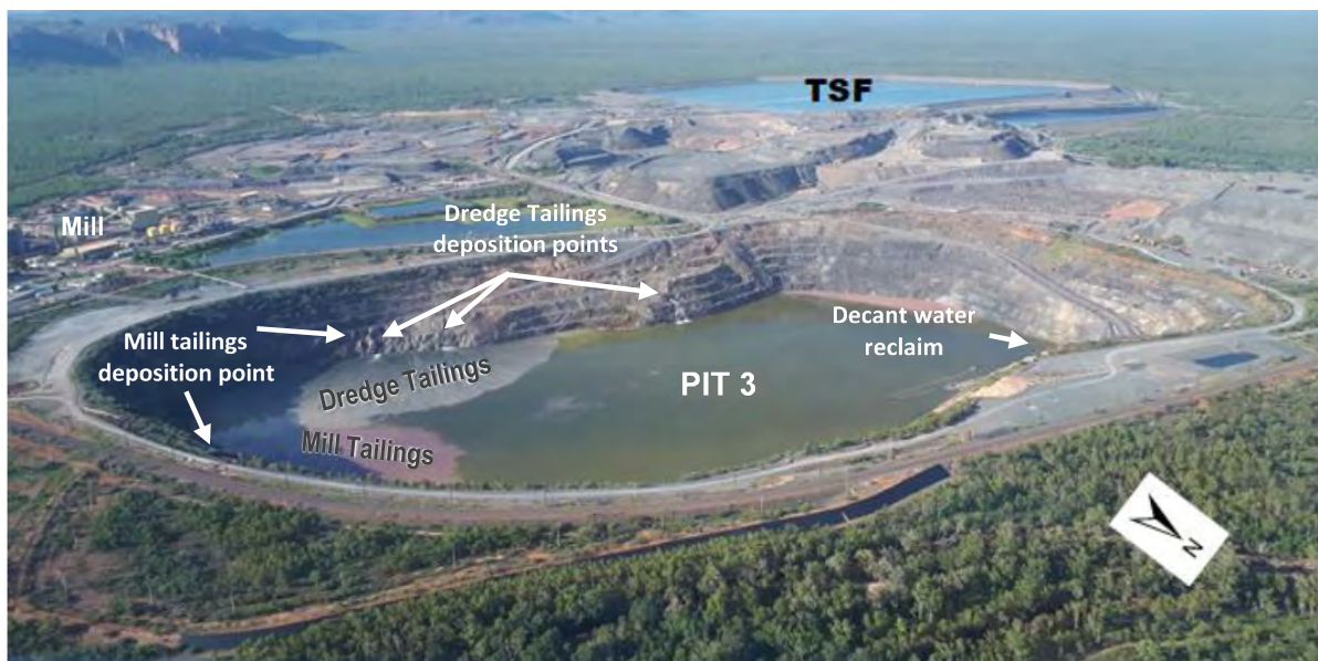
Figure 9-21: Pit 3 showing the original location of mill and dredge tailings deposition points
