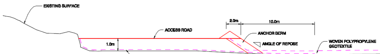
Figure 9-50 Typical geotextile anchor berm detail – section view
