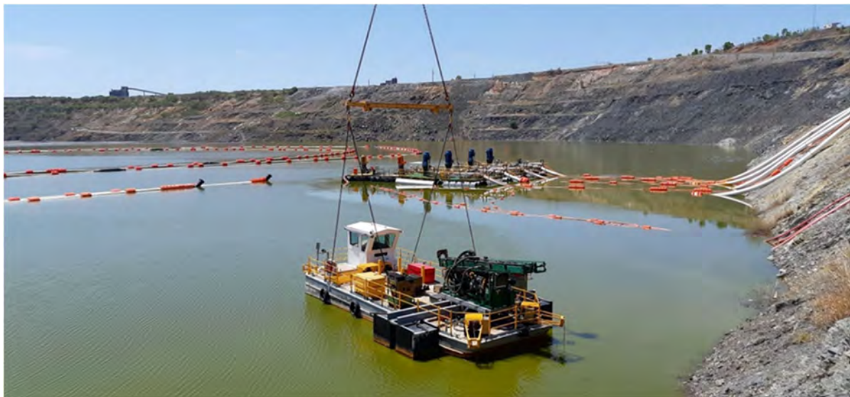
Figure 9-42 Placing CPTu barge in Pit 3 with CPTu rig mounted
