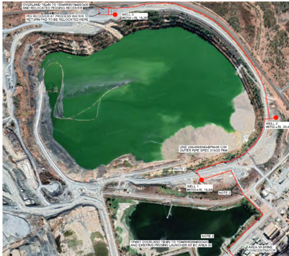
Figure 9-33 : Concept design for additional injection wells
