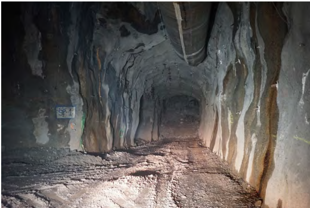
Figure 9-86: Picture taken 24 June after approx. 2,600 t of backfill has been placed in the decline (ERA 2022)
