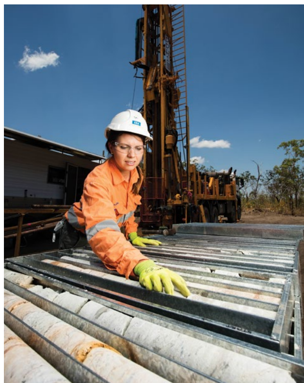
▲ Hydrogeologist Alana O'Neill inspects core drilled for groundwater monitoring bores
