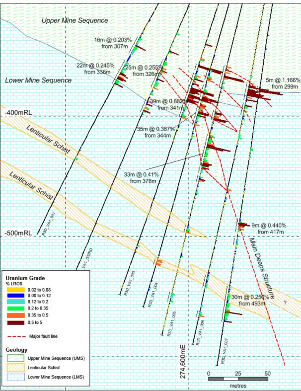
Figure 2 – Interpreted cross section showing the drilling results from cuddy VA1.
