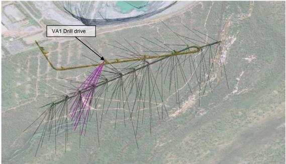
Figure 1 – Location of VA1 drilling from the first drill drive from the underground decline from which drilling has recently been completed (drill profiles shown in pink). Location of proposed underground drilling also shown from the underground decline (in grey).
