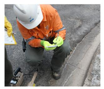
A Radiation Safety Advisor checks that the radiation dose levels of the material is well within safe levels
