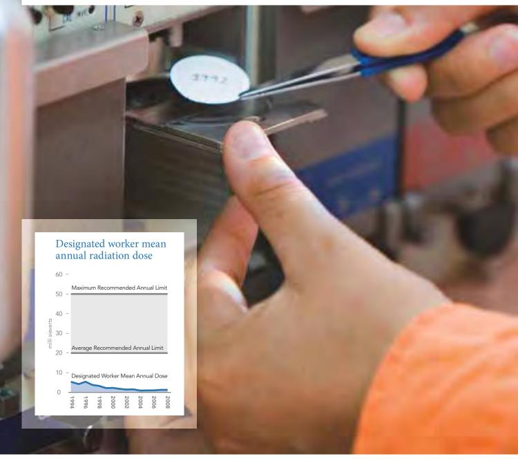
**Radiation monitoring:** Alpha Spectrometers are used to analyse dust filter pads from radiation monitoring equipment worn by designated ERA workers.
