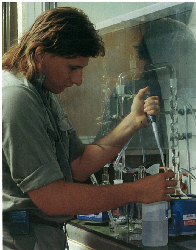
Technical Officer Ben Matthews carries out a distillation at Ranger's environment laboratory.
