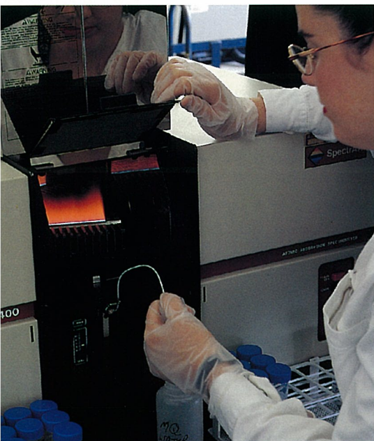
ANOTHER IMPORTANT USE OF URANIUM IS IN MEDICINE. PICTURED HERE IS A SPECTROMETER ANALYSIS USED IN PREPARING NUCLEAR PHARMACEUTICAL ISOTOPES.
