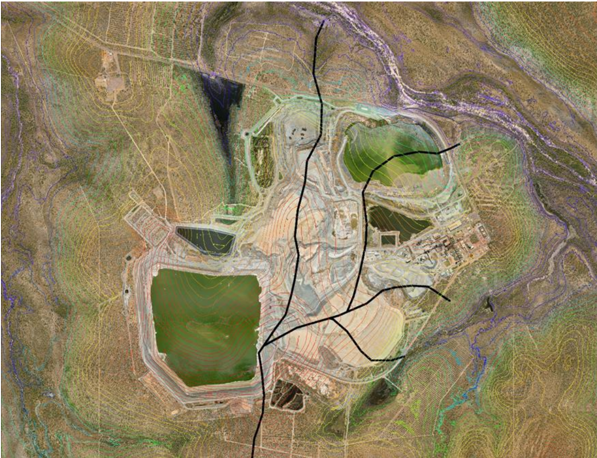
Figure 4-5: Preliminary plan for rocky outcrop habitat feature lines on the final landform
