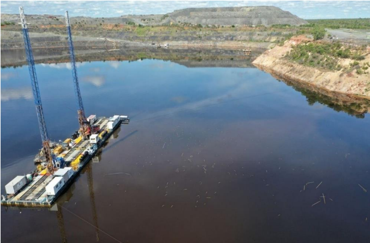
Plate 4-11: Pit 3 wicking barge and rigs
