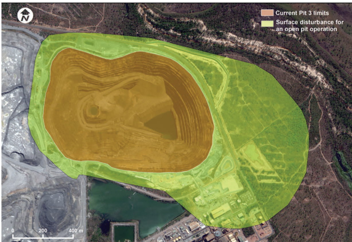
Projected surface disturbance required under an open pit mining scenario
